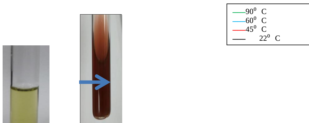
Figure-4. Color change from yellow color to brown due to formation of Silver nanoparticles.
